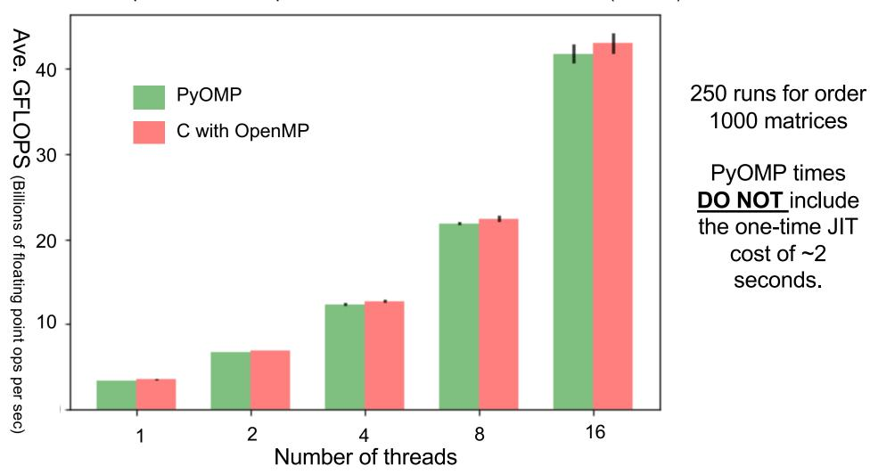
Intel® Xeon® E5-2699 v3 CPU, 18 cores, 2.30 GHz, threads mapped to a single CPU, one thread/per core, first 16 physical cores. Intel® icc compiler ver 19.1.3.304 (icc –std=c11 –pthread –O3 xHOST –qopenmp)
